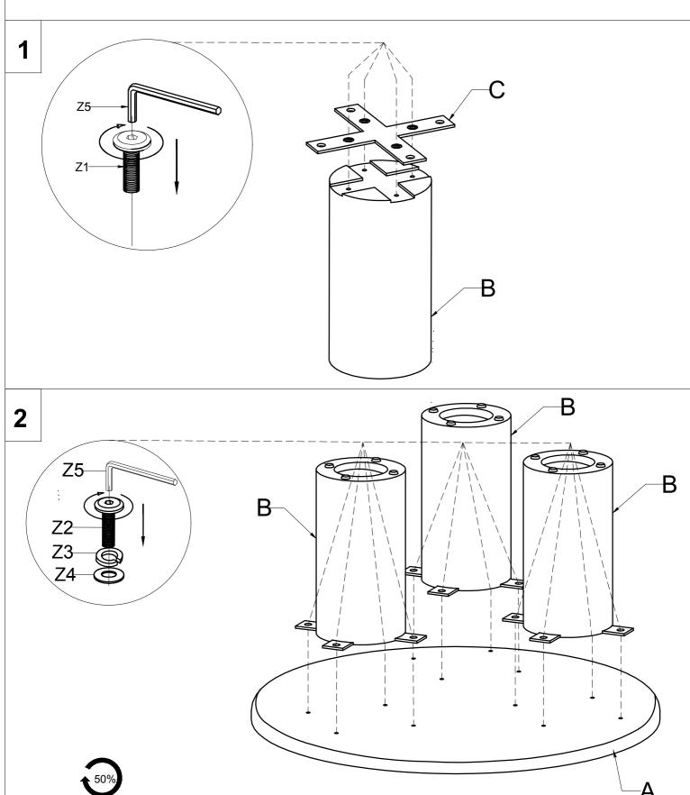
Tighten individual screw at 50%, and only fully tighten when screws are all in place.
