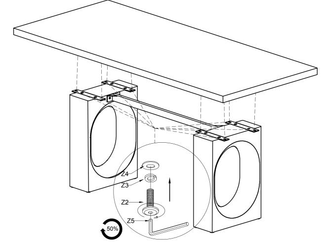
Tighten individual screw at 50%, and only fully tighten when screws are all in place.
